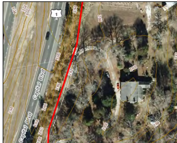
Figure 41: Enlarged section of tax parcel map depicting the slope of the NCDOT right-of-way on the east side of US 1
