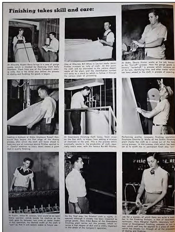
Figure 153: Steps in the finishing process, including “boil off” at upper right and beginning of dyeing, at center left, taking place in Wake Finishing Plant (source: Bur-Mil Review , July-August 1952)
